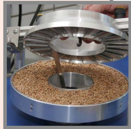
Shear cell of Ring Shear Tester RST-01.pc
