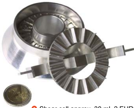
Shear cell approx. 30 ml, 2 EURO coin
